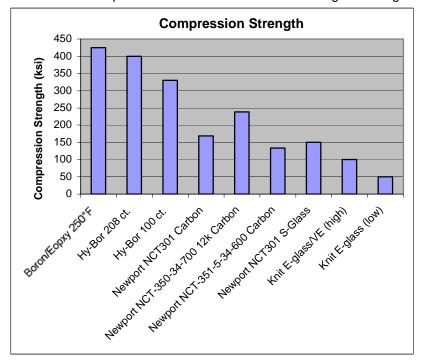
The first three products are Boron based showing their high compression strength. The next three are
