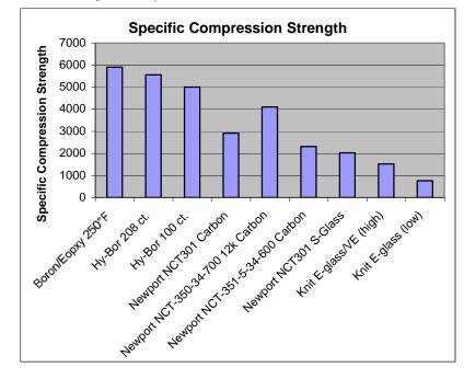
The "Specific Compression Strength" chart shows a similar trend to the "Compression Strength", with the carbon products looking better than the previous chart, because the carbon products have a lower density than the boron and glass based products.
